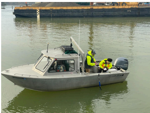
Crews collect water samples to confirm that dredging is conducted in compliance with water quality standards. (Geosyntec, 2026)
