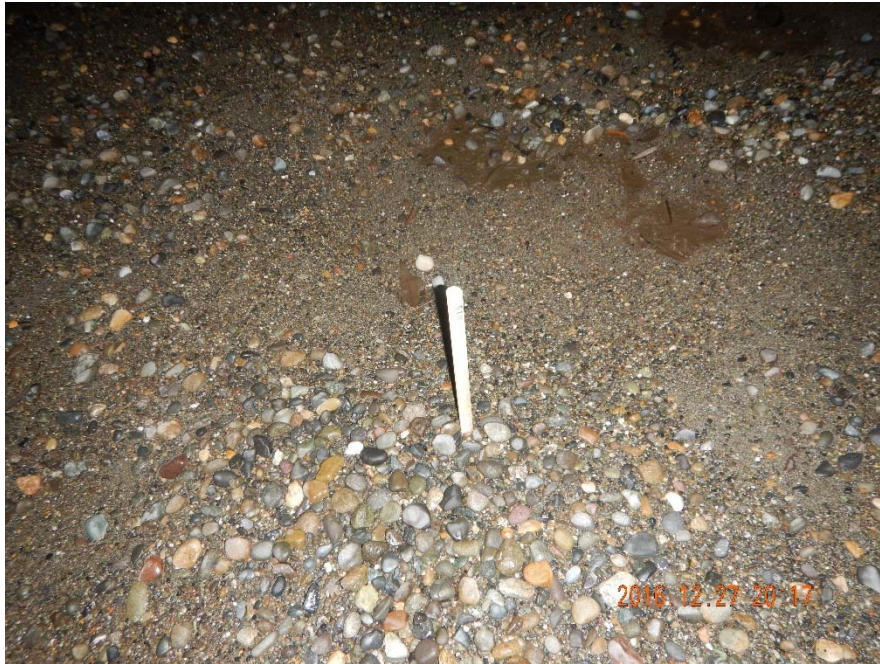
Photo 1-A: Typical grade stake observation at the Intertidal plot. This stake extends approximately 8 inches out of the gravelly sand.
