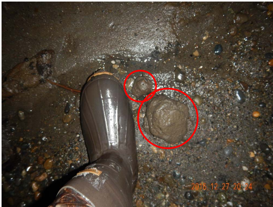
Photo 1-B: Undisturbed activated carbon balls (circled in red) were observed at the Intertidal plot during visual inspection.
